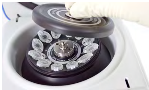
Built-in rotor MSR-12 and a protection lid
